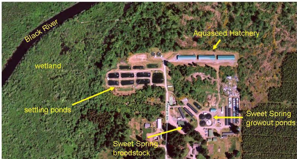
Figure 3. Schematic diagram of the Domsea Brood Stock Coho salmon farm in Rochester, Washington showing farm layout and proximity of settling ponds to the wetland and the Black River. This photo was taken before the construction of several new grow-out tanks (Google). The farm is classified as a flow-through system in this report. The broodstock and hatchery are operated in single-pass flow-through systems and the grow-out tanks reuse 85–98% of their water. By definition, this is a ‘closed’ system, and this farm is able to exert a high level of
